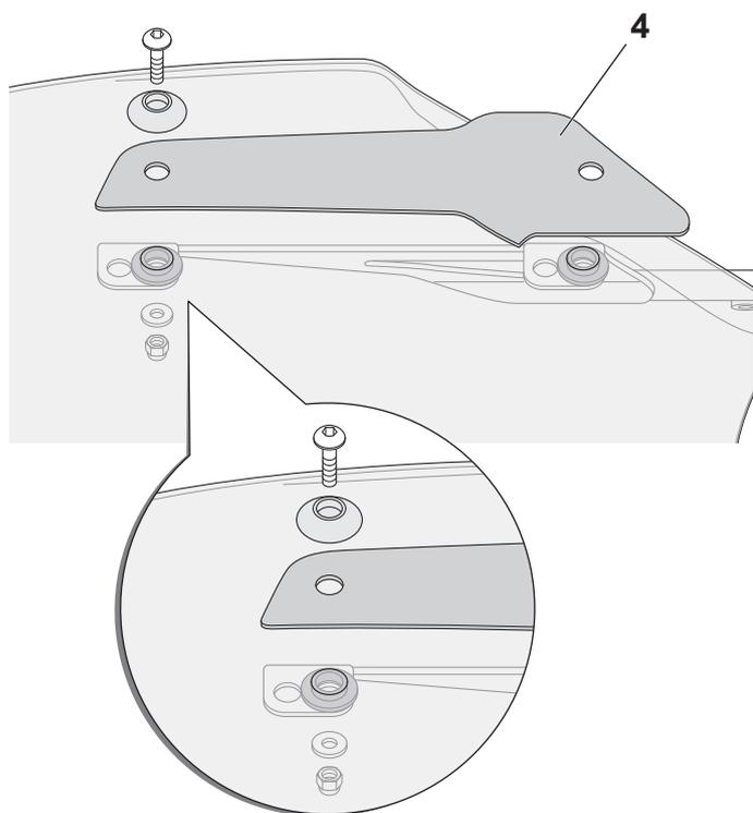
**GB** Position and definitely attach the left band (4) to the windscreen (top side) using a M6 screws, bushing, washer and blind nut (as in the figure).
