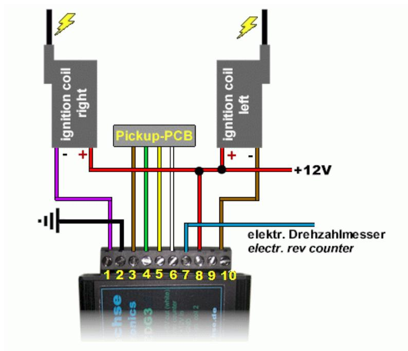
Ignition circuit diagram, contact breaker replacement
