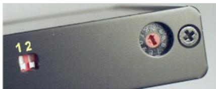
Figure 1 DIP switches and rotary switch.
