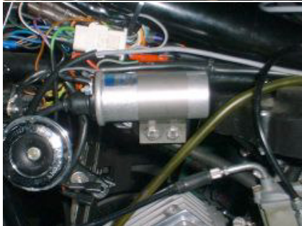
Mounting suggestion with Beru ZS220 coils
