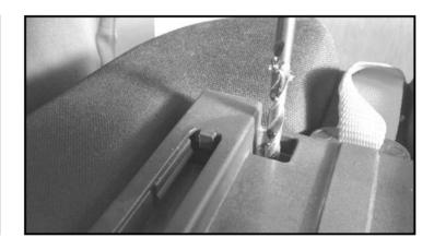
Bolting the lock unit on
