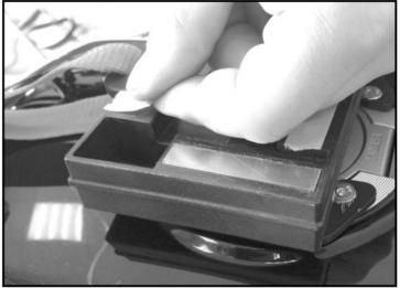
Control all screw connections after the assembling for tightness! Do not exceed the maximum load of 5 kg
