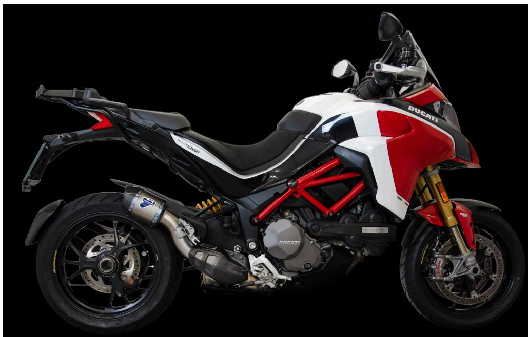
The homologated D193 system stands out for the compactness of its silencer complete with titanium sleeve and carbon fibre endcap; the 70mm link pipe and carbon fibre heat shield are finished with a titanium plate engraved with the Termignoni logo and the iconic "Pikes Peak edition". This system is compatible with the original side panniers and does not require any re-mapping of the ECU.
